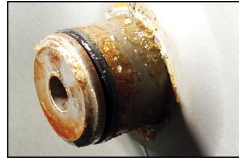
Replace the O-ring on the bottom of the filter pan. It must be in good shape and properly seated.
